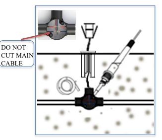
Step 5: Fix the luminaire to the sleeve by press.
