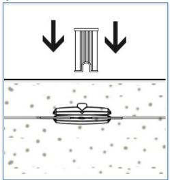
Step 3: Depending on tile thickness, raise the recessed sleeve by 1-2cm above the surface. Connect the luminaire input cable to the main supply (180-250V AC, 50/60Hz) using a waterproof KIT.
