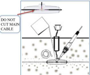
• Step 5: Fix the luminaire to the sleeve by press.
