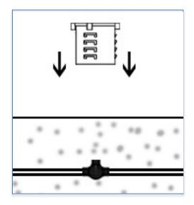
• **Step 3**: Depending on tile thickness, raise the recessed sleeve by 1-2cm above the surface. Connect the luminaire input cable to the main power supply (12V) cable.
