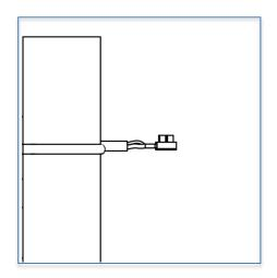
Step 2: Connect the luminaire power cable to the main supply using terminal blocks or connectors. Wrap
