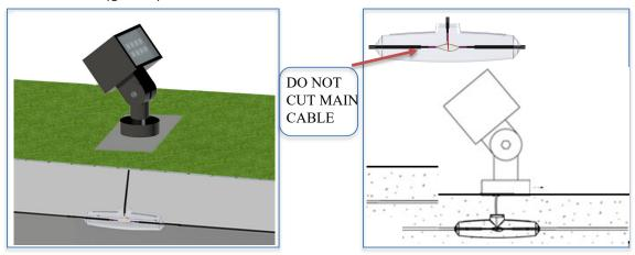
Step 5: Solder & Wrap the connections with 3M waterproof tape & electrical tape. Fill the M11 kit with epoxy as illustrated.
