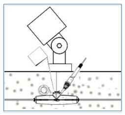
Step 6: Install the luminaire body to the bottom plate of the luminaire and adjust the luminaire angle by allen key as illustrated.
