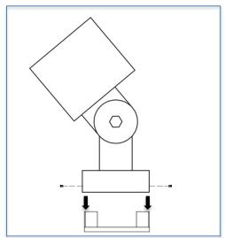
Step 3: : Mount the bottom plate of the luminaire onto a hard surface using appropriate stainless steel screws as illustrated.
