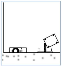
• Step 3: : Connect the luminaire input cable to the main power supply (24VDC) cable. Ensure the junction box is installed within one meter from the luminaire. (Do not cut the main power supply cable, just remove insulation, twist the luminaire input cable around the main cable). Solder the connections, wrap the connection with 3M waterproof tape & electrical tape and keep all the connections inside the junction box as illustrated.
