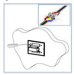
• Step 5: Fix the diffuser on the luminaire electrical compartment using screws.
