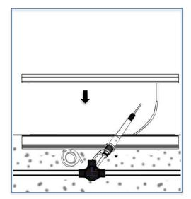
• Step 5: Fix the luminaire to the sleeve by press
