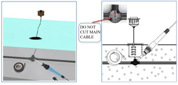
• Step 5: Fix the luminaire to the sleeve by provided screws as illustrated.
