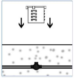
• Step 3: Depending on tile thickness, raise the recessed sleeve by 1-2cm above the surface. Connect the luminaire input cable to the power supply cable.
