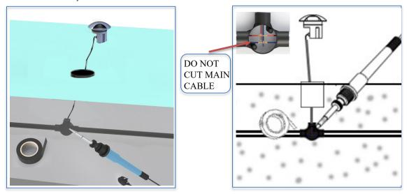
Step 5: Fix the luminaire to the sleeve by press as illustrated.
