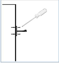
Step 3: Connect the luminaire power cable to the mains supply using terminal blocks or connectors. Wrap connectors or terminal blocks with Waterproof electrical tape. Please make sure the earth (ground) wire is reliable as illustrated
