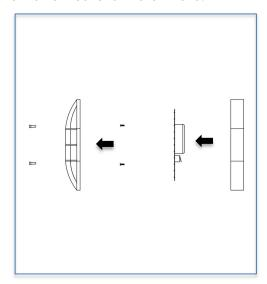
• Step 3: : Mount the back body on to a hard surface using provided screws as illustrated.
