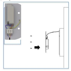
• Step 5: Reinstall the front cover back on to the luminaire as illustrated.
