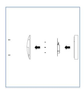
• Step 3: : Mount the back body on to a hard surface using provided screws as illustrated.
