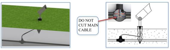
• Step 8: Solder the connections, wrap the connection with 3M waterproof tape & electrical tape and keep all the connections inside the junction box. Put silicon on the top surface of the junction box and close the junction box with screws as illustrated.
