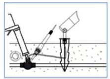
• Step 9: Adjust the luminaire angle by thumb nut as illustrated.
