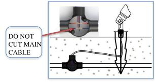
• Step 5: Solder the connections, wrap the connection with 3M waterproof tape & electrical tape and keep all the connections inside the junction box and put silicon on the top surface of the junction box and close the junction box with screws as illustrated.
