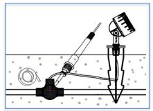
• Step 6: Adjust the luminaire angle by thumb nut as illustrated.
