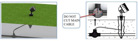
• Step 5: Solder the connections, wrap the connection with 3M waterproof tape & electrical tape and keep all the connections inside the junction box and put silicon on the top surface of the junction box and close the junction box with screws as illustrated.
