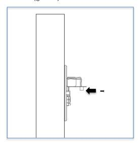
Step 3: Fix the Outer cover using an Allen Key
