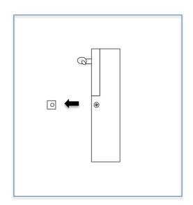
Step 3: Take out the power supply from the wall where luminaire has to be installed. Fix fishers on the wall for the mounting bracket
