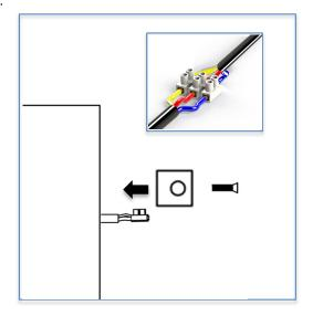
• Step 5: Connect the luminaire to power supply using connectors and wrap connection using 3M tape.
