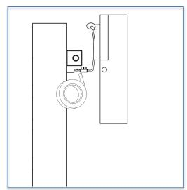
Step 6: Mount the luminaire on the bracket using screws.
