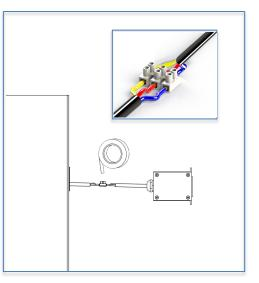
• Step 5: Fix the luminaire to the sleeve by press, then screw in the outer plate.
