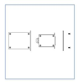
• Step 2: Dig the mounting hole 20cm deeper before installing the Sleeve. Install the sleeve in the wall depending on type of tile thickness or concrete, raise the sleeve by 1-2cm above the surface.
