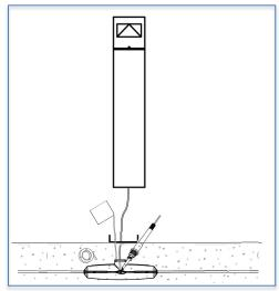
• Step 6: Install the luminaire body to the bottom plate of the luminaire as illustrated.
