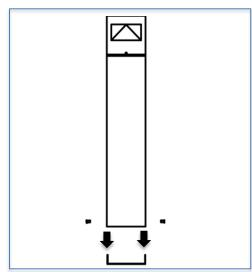
• **Step 3:** Mount the bottom plate of luminaire onto a hard surface using appropriate stainless steel screws as illustrated. Maintain foundation height 50mm above the ground for softscape installation.
