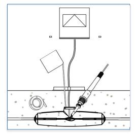
• Step 6: Install the luminaire body to the bottom plate of the luminaire as illustrated.
