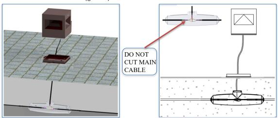
• **Step 5**: Solder & Wrap the connections with 3M waterproof tape & electrical tape. Fill the M11 kit with epoxy as illustrated.
