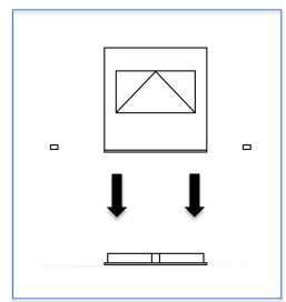
• **Step 3:** Mount the bottom plate of luminaire onto a hard surface using appropriate stainless steel screws as illustrated. Maintain foundation height 50mm above the ground for softscape installation.
