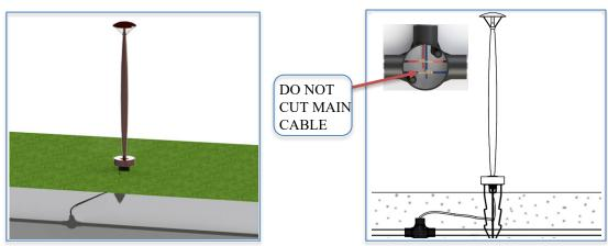
**Step 5:** Solder the connections, wrap the connection with 3M waterproof tape & electrical tape and keep all the connections inside the junction box and put silicon on the top surface of the junction box and close the junction box with screws as illustrated.
