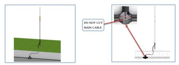
• Step 5: Solder the connections, wrap the connection with 3M waterproof tape first and then electrical tape and keep all the connections inside the junction box and put silicon on the top surface of the junction box and close the junction box with screws as illustrated.
