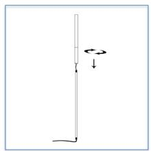
Step 3: Fix the luminaire stem onto the stake by rotating after inserting the cable inside the stake hole. Make sure the luminaire input cable is rotating with the luminaire stem to avoid potential damage to the luminaire input cable as illustrated. Depending on type of surface raise the stake by 5cm above the surface as illustrated.
