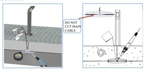
**Step 5:** Mount the luminaire onto a hard surface using appropriate stainless steel screws as illustrated. Maintain foundation height 50mm above the ground for softscape installation.
