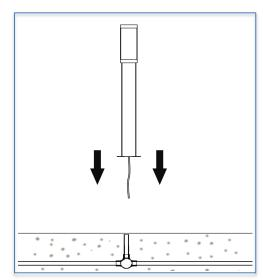
Step 2: : Connect the luminaire input cable to the main power supply (12V) cable.
